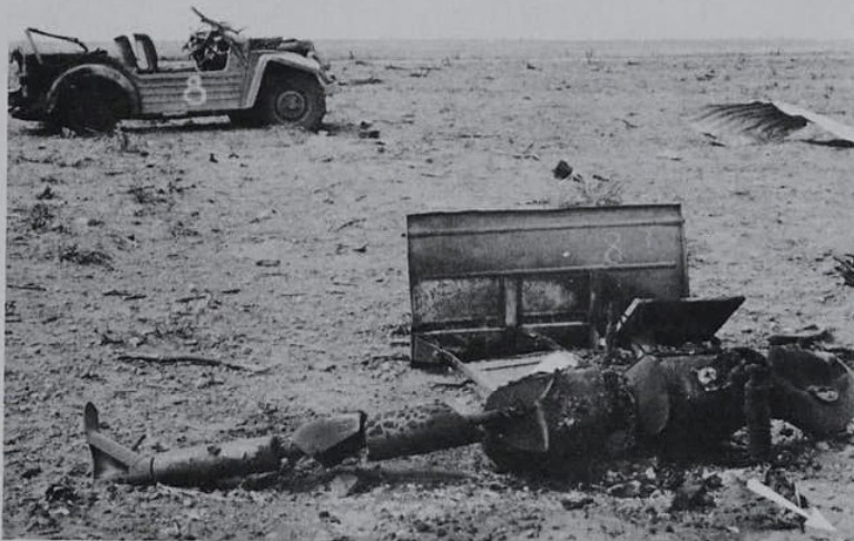
FIGURE 18. ROUND 3. DUMMY PASSENGER FROM CHAMP SIDEWAYS TO BLAST AT 2825 ft BURNT OUT AND WITH ONE LEG MISSING
